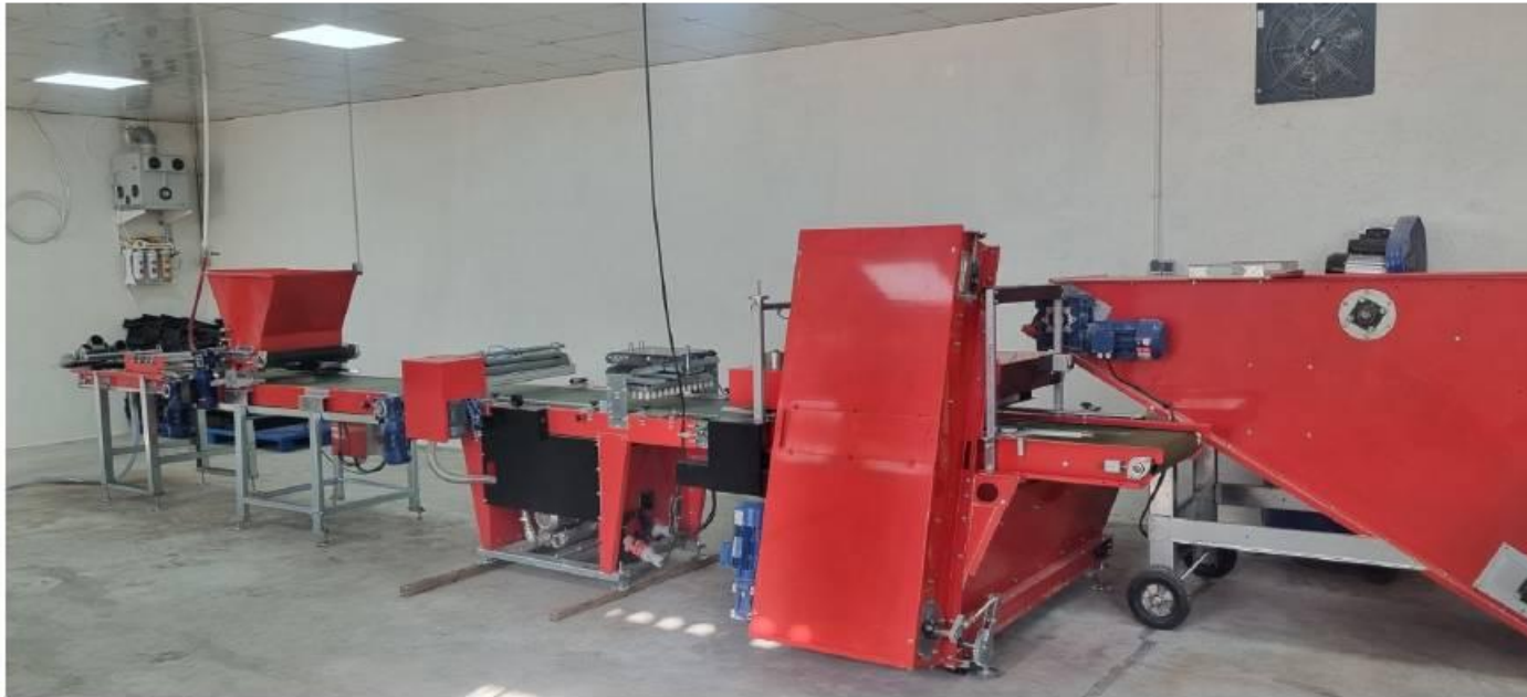
Automated seed-sowing line
